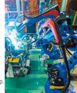
Automated welding equipment
